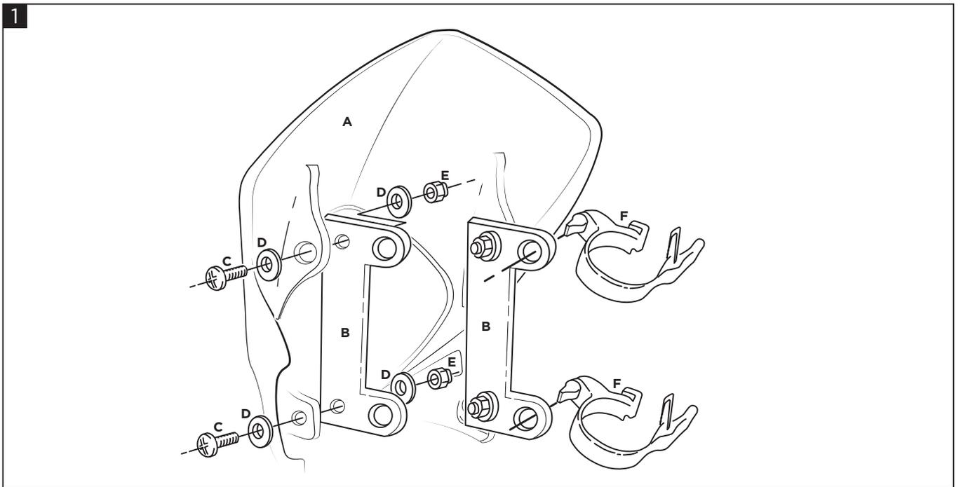
**How to mount the headlight using the spacer plates provided in the mounting kit: Apply the spacer plates (B) to the headlight using the screws (C), the washers (D), and the nuts (E) provided in the kit. Fasten the plates (B) to the moto using the bands (F) as illustrated in the figure.**
